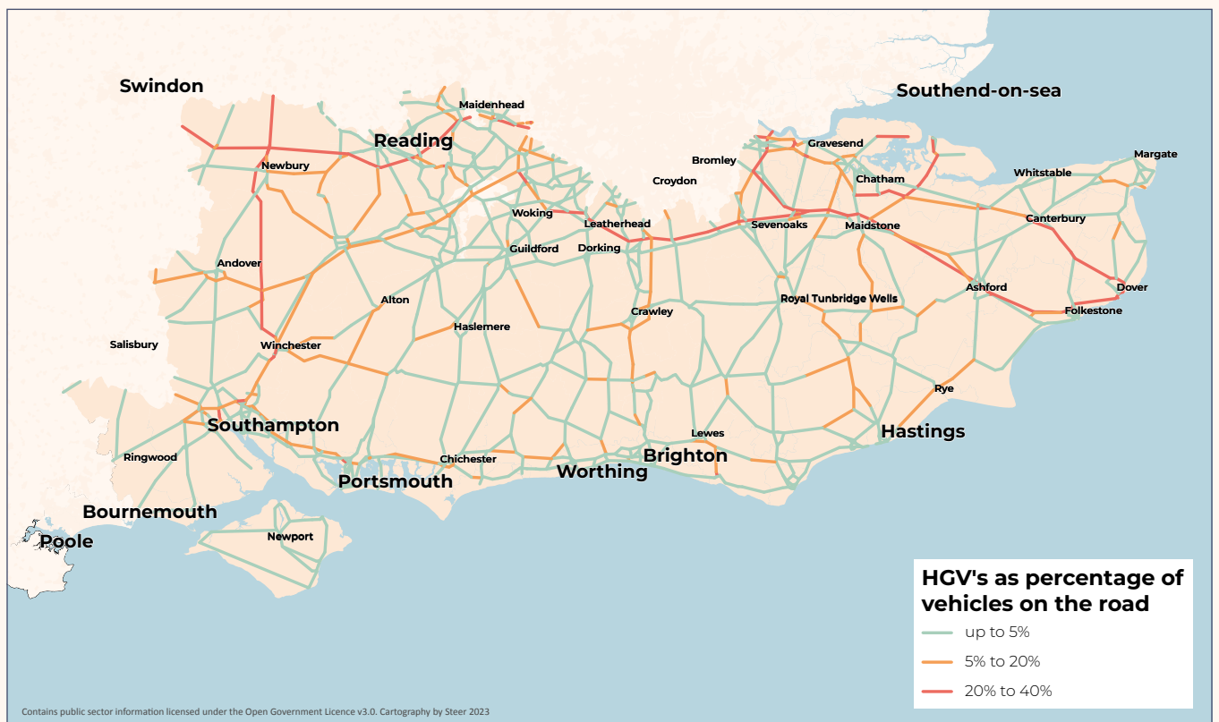
Figure 2.11: HGVs as a Percentage of Vehicles on the Road Source: DfT Traffic Counts and Steer Analysis
